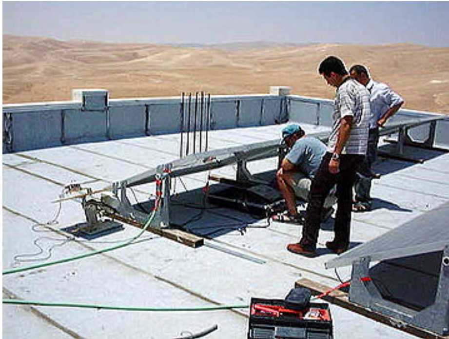
Figure 3: The process of I-V curve measurement for module “H”. The plane-of-array pyranometer is seen on the left of the picture.
